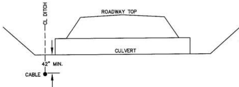
CABLE SHALL BE 42" (MINIMUM) BELOW CULVERT FLOW LINE AT ALL CULVERTS WHERE CABLE IS PLACED AROUND THE END OF CULVERT.
