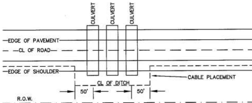
TYPICAL DETAIL OF THE PLACEMENT OF CABLE AROUND CULVERTS
